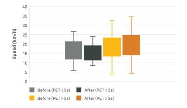
After Curb Radius Reduction, the Speed of Turning Vehicles Involved in a Conflict (With Pet Less Than or Equal 3 Seconds) Dropped:
